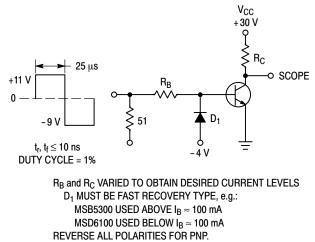
Figure 2. Switching Time Test Circuit
