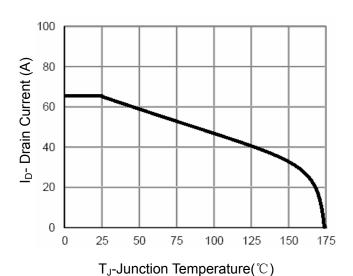
**Figure 10 ID Current- Junction Temperature**
