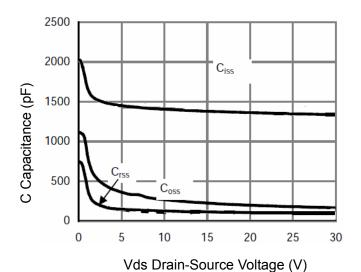
Figure 7 Capacitance vs Vds
