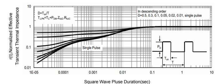
Figure 11 Normalized Maximum Transient Thermal Impedance
