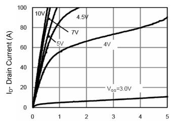
Vds Drain-Source Voltage (V)
