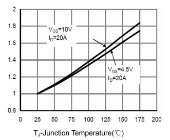
Figure 4 Rdson-JunctionTemperature
