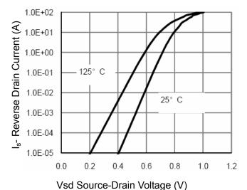
Figure 6 Source- Drain Diode Forward
