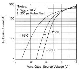
Figure 2. Transfer Characteristics
