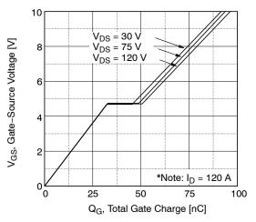
Figure 6. Gate Charge Characteristics
