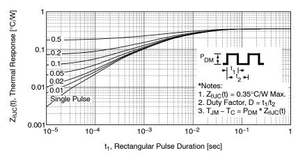
Figure 12. Transient Thermal Response Curve
