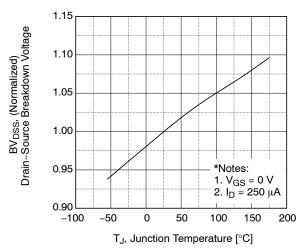
Figure 7. Breakdown Voltage Variation vs. Temperature
