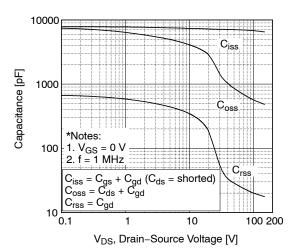
Figure 5. Capacitance Characteristics
