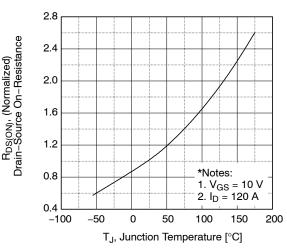
Figure 8. On–Resistance Variation vs. Temperature
