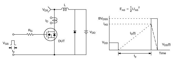
Figure 15. Unclamped Inductive Switching Test Circuit & Waveforms
