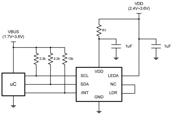
STK3311-WV Typical Application Circuit with Only One Supply Voltage
