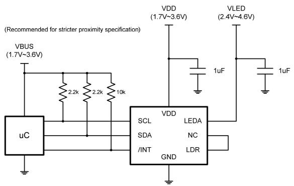
STK3311-WV Typical Application Circuit with Independent VDD and VLED Supply Voltage
