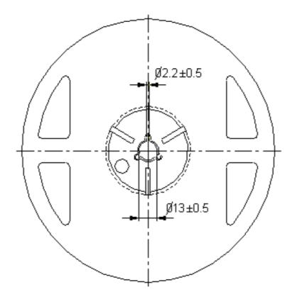
Note: 01. The tolerance unless mentioned is ±0.1mm 02. The measured unit is "mm"
