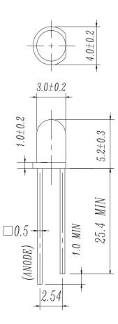
Note: Tolerances unless dimensions ±0.25mm
