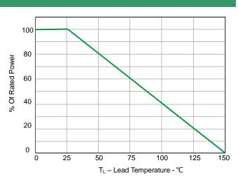
Fig 2. Power Derating Curve
