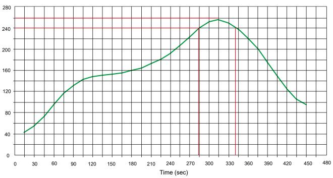
Peak Temp=257°C, Ramp Rate=0.802deg. °C/sec
