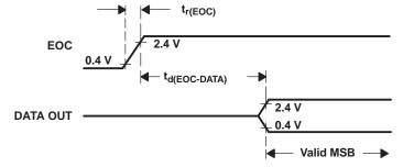
Figure 8. EOC and DATA OUT Voltage Waveforms
