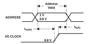
Figure 4. ADDRESS Setup and Hold Time Voltage Waveforms
