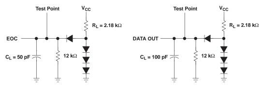
Figure 2. Load Circuits
