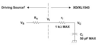
V<sub>I</sub> = Input Voltage at A0-A10
