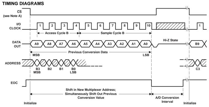
A. To minimize errors caused by noise at  $\overline{CS}$ , the internal circuitry waits for a setup time plus two falling edges of the internal system clock after  $\overline{CS}$ ↓ before responding to control input signals. Therefore, no attempt should be made to clock in an address until the minimum  $\overline{CS}$  setup time has elapsed.
