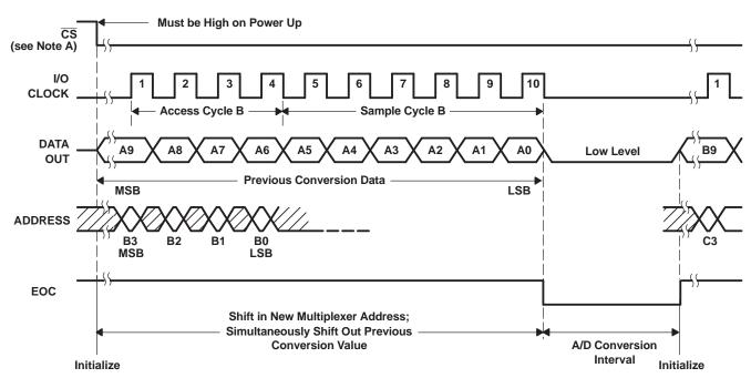
A. To minimize errors caused by noise at CS, the internal circuitry waits for a setup time plus two falling edges of the internal system clock after CS↓ before responding to control input signals. Therefore, no attempt should be made to clock in an address until the minimum CS setup time has elapsed.
