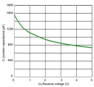
Fig 4. Capacitance vs. Reveres voltage
