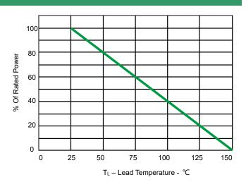
Fig 2.Power Derating Curve
