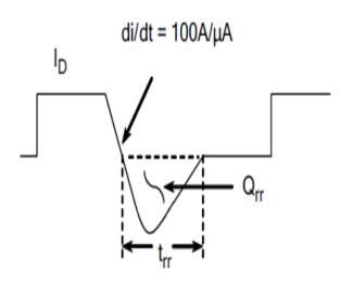
Figure 16. Diode Reverse Recovery Waveform
