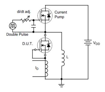
Figure 15. Diode Reverse Recovery
