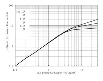
Figure 2. Typical Transfer Characteristics
