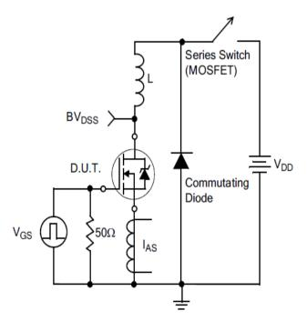
Figure 17. Unclamped Inductive Switching Test Circuit
