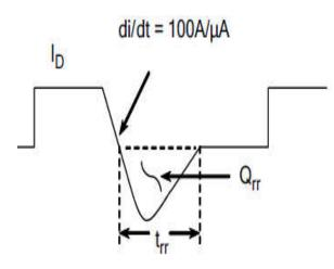
Figure 16. Diode Reverse Recovery
