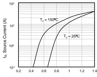
Figure 2. Body Diode Forward Voltage
