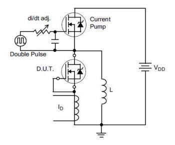
Figure 15. Diode Reverse Recovery
