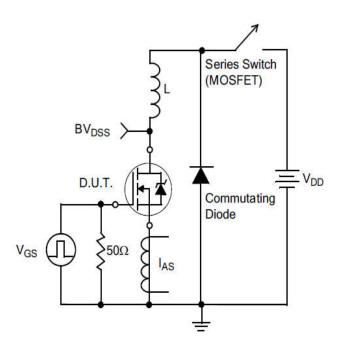
Figure 17. Unclamped Inductive Switching Test Circuit
