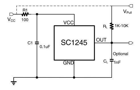
The SC1245 contains an on-chip voltage regulator and can operate over a wide supply voltage range. In applications that operate the device from an unregulated power supply, transient protection must be added externally. For applications using a regulated line, EMI/RFI protection may still be required. R1 is for improved CI performance, and could be 100 or 200  $\Omega$  typically.
