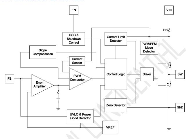
Figure 2. MT3410LB Block Diagram
