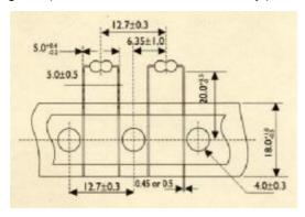
PN Type Forming for Taping (rated watts from 1/4W to 2WS applicable only )
