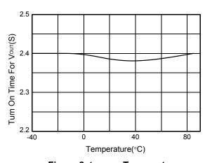
Figure 8.  $t_{VON}$  vs. Temperature
