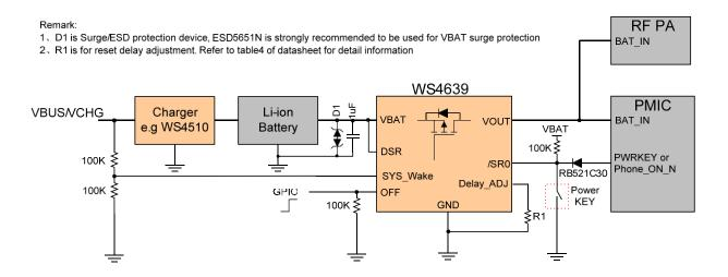
Figure 1. Typical Application without power path system
