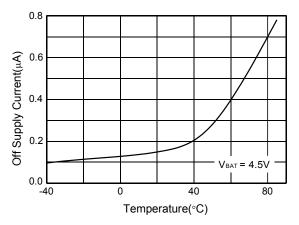
Figure 4. Off Supply Current vs. Temperature
