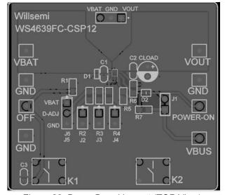
Figure 22. Demo Board Layout (TOP View)
