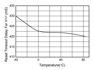
Figure 10.  $t_{\text{REC1}}$  vs. Temperature
