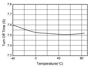
Figure 7. t<sub>OFF</sub> vs. Temperature
