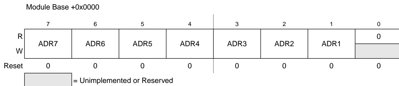
Figure 10-3. IIC Bus Address Register (IBAD)
