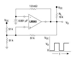
Figure 10. Free-Running Square-Wave Oscillator
