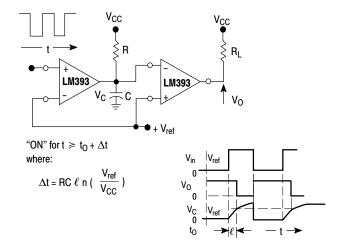
Figure 11. Time Delay Generator
