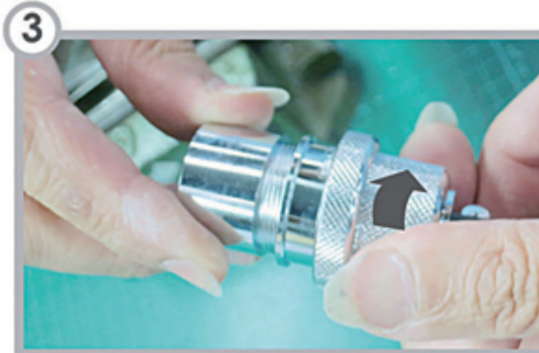
3 本體與上固定體對鎖，將螺紋順時針方向鎖緊（需轉動本體鎖入，非轉動接頭） The body and the upper one are locked together. Screw clockwise and be sure to only rotate the body itself instead of the whole connector
