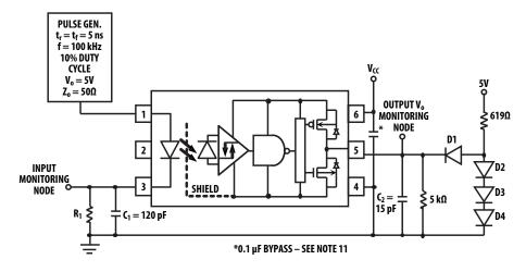
THE PROBE AND JIG CAPACITANCES ARE INCLUDED IN C1 AND C2.
