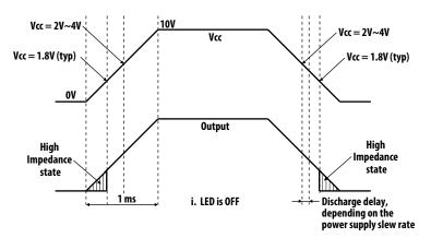
Figure 11  $\,V_{CC}$  Ramp When LED OFF
