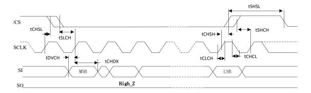
Figure 47. Output Timing
