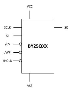
Figure 2. Pin Configuration SOP 208 mil
