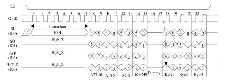
Figure 19. Quad I/O word Fast Read Sequence Diagram (Previous command set (M5-4) =(1,0))
