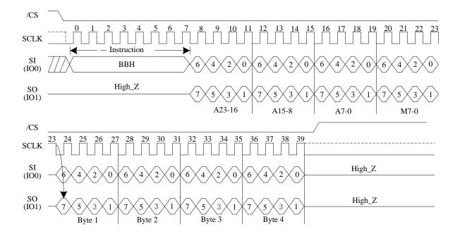
Figure 15. Dual I/O Fast Read Sequence Diagram (Previous command set (M5-4) =(1,0))
