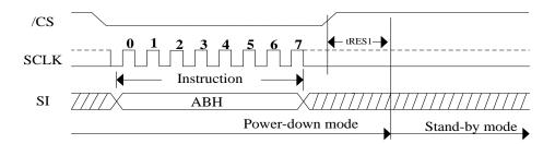
Figure 26.b. Release Power-down Instruction (QPI Mode)
