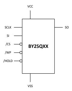
Figure 2. Pin Configuration SOP8
