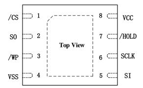
Figure 3.2. Pin Configuration DFN 2\*3mm
