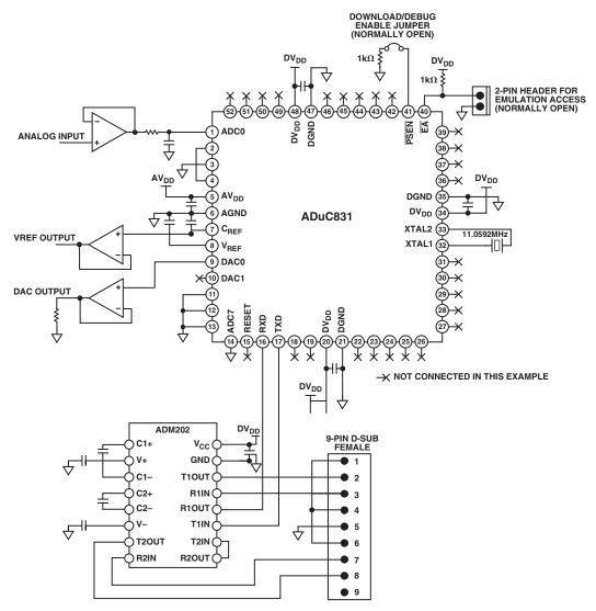
Figure 64. Example ADuC831 System (PQFP Package)
