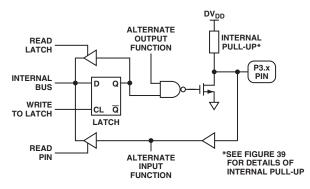
Figure 40. Port 3 Bit Latch and I/O Buffer
