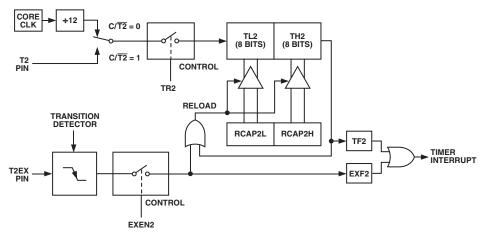
Figure 49. Timer/Counter 2, 16-Bit Autoreload Mode
