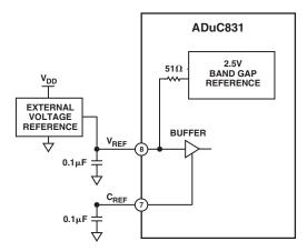
Figure 13. Using an External Voltage Reference
