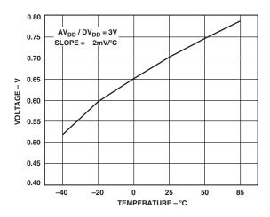
*TPC 16. Typical Temperature Sensor Output vs. Temperature*
