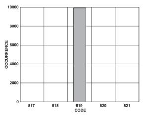
TPC 9. Code Histogram Plot,  $V_{DD} = 5 V$
