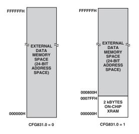
Figure 4. Internal and External XRAM
