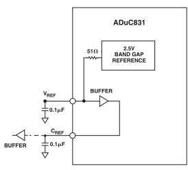
Figure 11. Decoupling V<sub>REF</sub> and C<sub>REF</sub>
