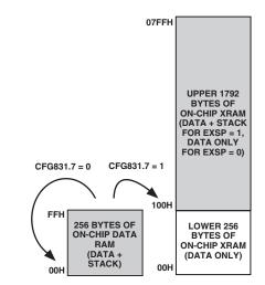
Figure 3. Extended Stack Pointer Operation
