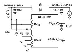
Figure 60. External Dual-Supply Connections
