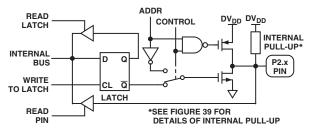
Figure 38. Port 2 Bit Latch and I/O Buffer
