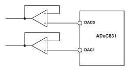
Figure 25. Buffering the DAC Outputs
