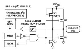
Figure 42. SCLOCK Pin I/O Functional Equivalent in I<sup>2</sup>C Mode
