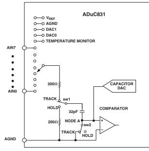
Figure 9. Internal ADC Structure
