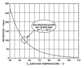
Figure 18. Flash/EE Memory Data Retention
