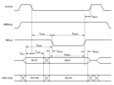
Figure 72. External Data Memory Write Cycle
