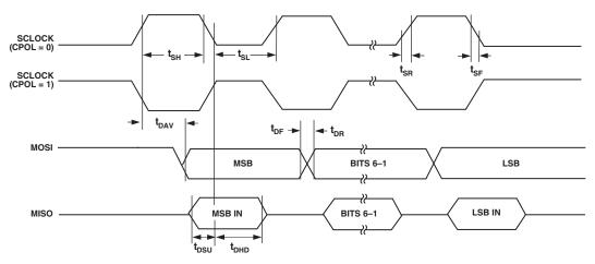
Figure 75. SPI Master Mode Timing (CPHA = 1)
