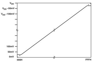
Figure 22. Endpoint Nonlinearities Due to Amplifier Saturation
