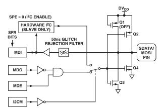
Figure 44. SDATA/MOSI Pin I/O Functional Equivalent in I<sup>2</sup>C Mode
