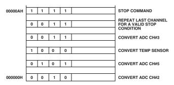
Figure 14. Typical DMA External Memory Preconfiguration
