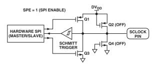
Figure 41. SCLOCK Pin I/O Functional Equivalent in SPI Mode
