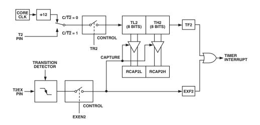
Figure 50. Timer/Counter 2, 16-Bit Capture Mode
