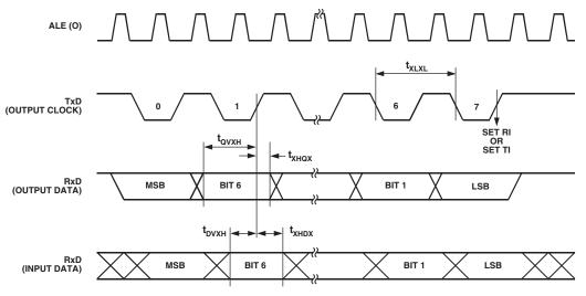
Figure 73. UART Timing in Shift Register Mode
