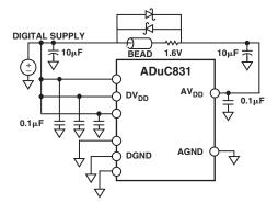
Figure 61. External Single-Supply Connections
