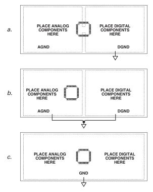
Figure 63. System Grounding Schemes
