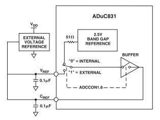
Figure 12. Using an External Voltage Reference
