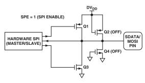
Figure 43. SDATA/MOSI Pin I/O Functional Equivalent in SPI Mode
