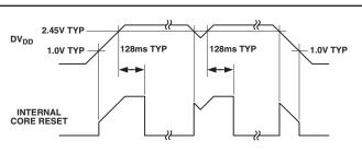
Figure 62. Internal POR Operation
