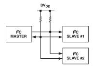
Figure 34. Typical I<sup>2</sup>C System
