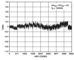
TPC 1. Typical INL Error,  $V_{DD} = 5 V$
