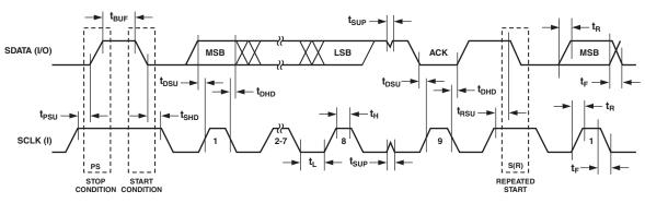
Figure 74. I<sup>2</sup>C Compatible Interface Timing
