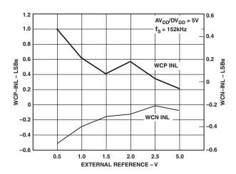
TPC 3. Typical Worst Case INL Error vs.  $V_{REF_r}$ ,  $V_{DD}$  = 5 V
