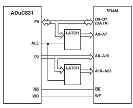
Figure 59. External Data Memory Interface (16 MBytes Address Space)
