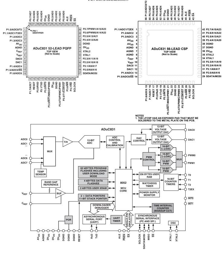
Figure 1. ADuC831 Block Diagram (Shaded areas are features not present on the ADuC812)
