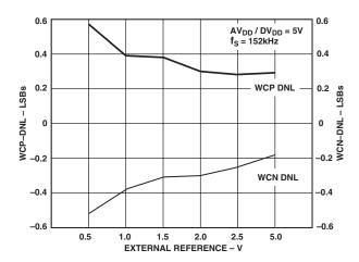
TPC 7. Typical Worst Case DNL Error vs.  $V_{REF}$ ,  $V_{DD} = 5 V$
