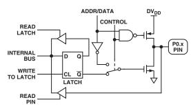
Figure 36. Port 0 Bit Latch and I/O Buffer
