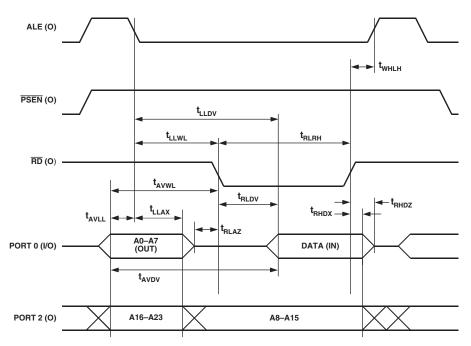
Figure 71. External Data Memory Read Cycle
