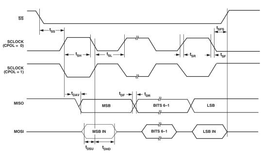
Figure 77. SPI Slave Mode Timing (CPHA = 1)
