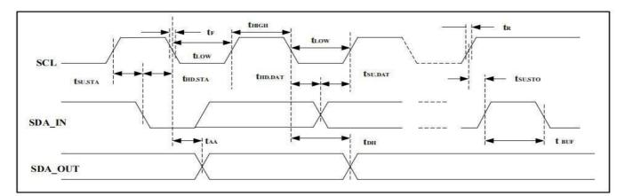
Figure 11. SCL: Serial Clock, SDA: Serial Data I/O
