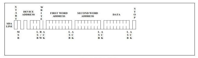
Figure 6. Byte Write
