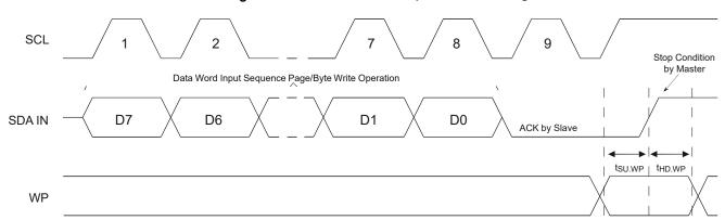
Figure 5-5. Write Protect Setup and Hold Timing
