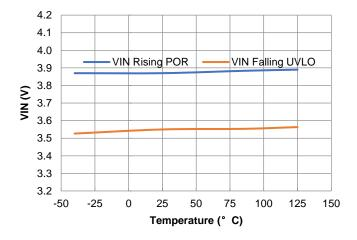
Figure 5. UVLO Vs. Temperature
