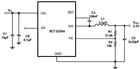
Figure 8. 12V Input, 3.3V/3A Output
