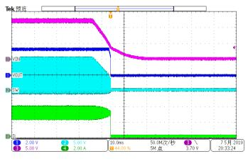
Figure 12. Power Down VIN=12V, VOUT=3.3V, IOUT=3A
