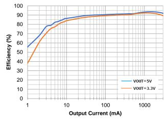
Figure 1. SCT2230A Efficiency, Vin=12V
