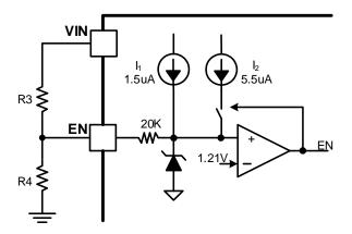
Figure 7. Adjustable VIN UVLO
