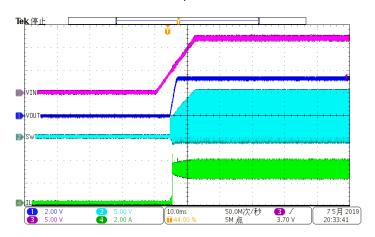
Figure 11. Power Up VIN=12V, VOUT=3.3V, IOUT=3A
