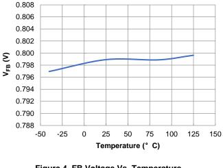
Figure 4. FB Voltage Vs. Temperature
