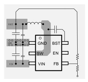
Figure 15. PCB Layout Example
