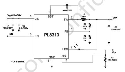
Work Mode 1: CS to GND with sensing resistor or short to GND directly Fig.18 Schematic
