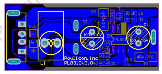
C2, C6, C9 are optional, R6, C4 are used to improve EMI only Fig.19 PCB Layout
