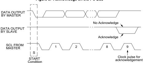
Figure 5. Acknowledge on the I<sup>2</sup>C Bus
