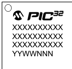
121-Lead TFBGA (10x10x1.1 mm)
