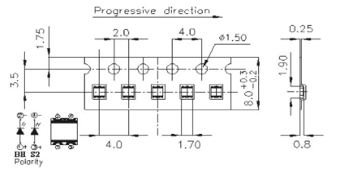
Note: The tolerances unless mentioned is ±0.1mm ,Unit = mm **Moisture Resistant Packaging**
