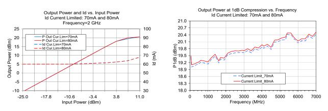
Fig 2. Output Power and Id vs. Input Power and Frequency.
