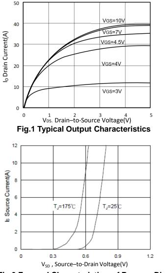
Fig.3 Forward Characteristics of Reverse Diode
