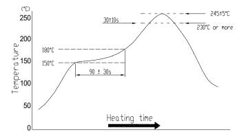
Temperature profile for reflow soldering
