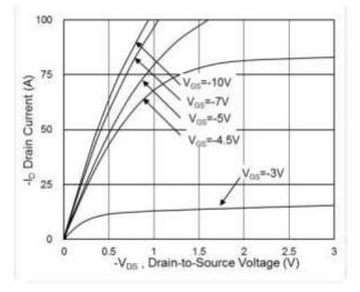
Fig.1 Typical Output Characteristics
