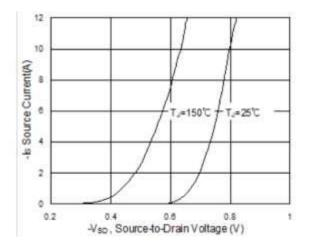
Fig.3 Forward Characteristics of Reverse Diode Fig.4 Gate-Charge Characteristics
