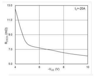
Fig.2 On-Resistance vs. G-S Voltage
