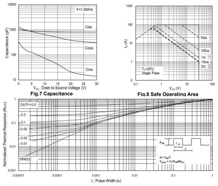
Fig.9 Normalized Maximum Transient Thermal Impedance
