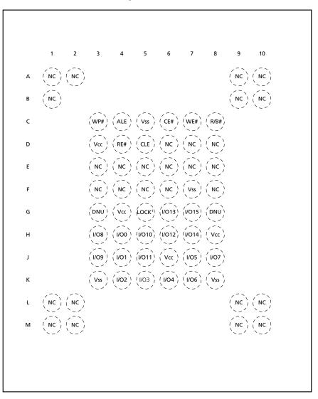
Note: 1. For the 3V device, G5 changes to DNU. NO LOCK function is available on the 3.3V device.
