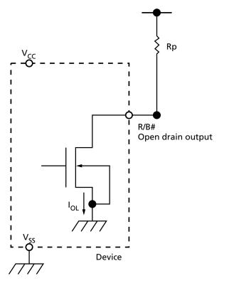
Figure 17: <sup>t</sup>Fall and <sup>t</sup>Rise (3.3V V<sub>CC</sub>)
