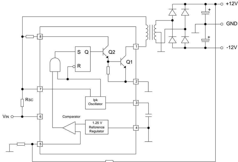
Higher Output Power, Higher Input Voltage
