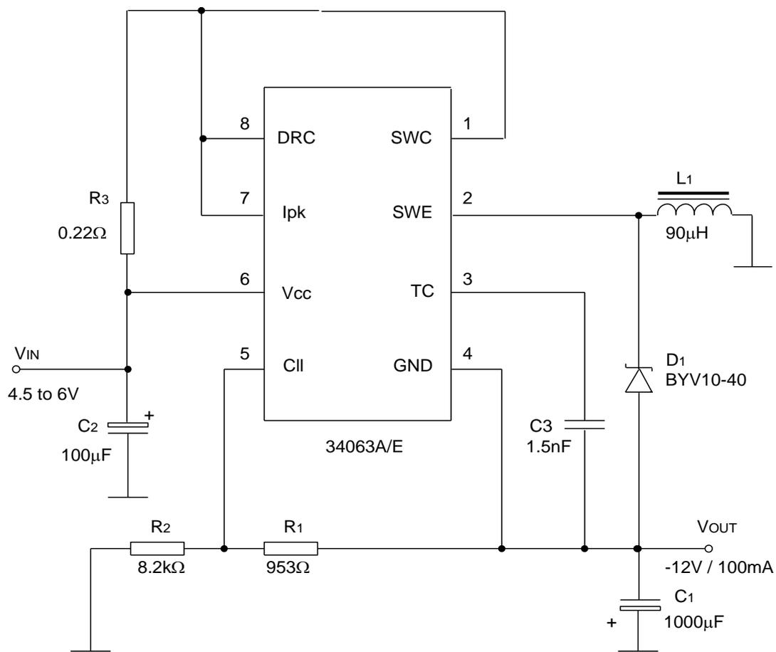
Test Condition ( $V_{OUT} = -12\text{ V}$ )
