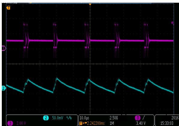
V_{IN}=3.6V, I_{OUT}=0.1A Ripple Waveform
