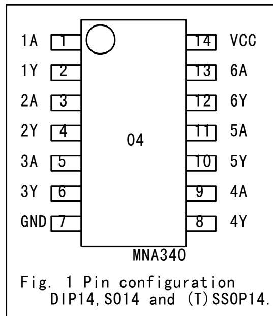
Fig. 1 Pin configuration
