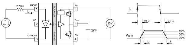
Figure 17.  $I_F$  to  $V_{OUT}$  Propagation Delay, Rise Time and Fall Time
