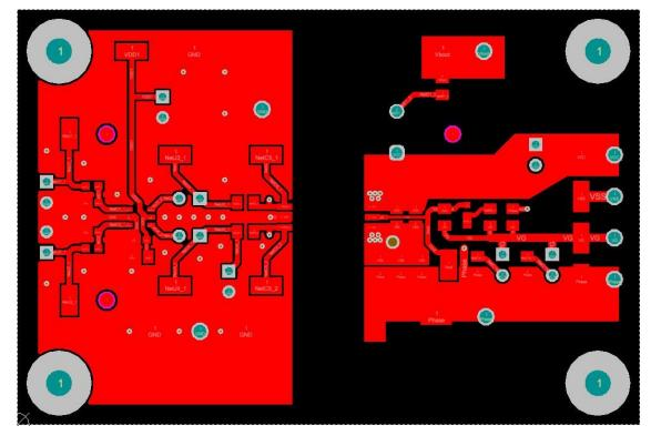
Figure 31. Top-Layer Traces and Copper
