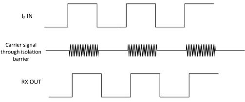
Figure 21. On-Off Keying (OOK) Based Modulation Scheme
