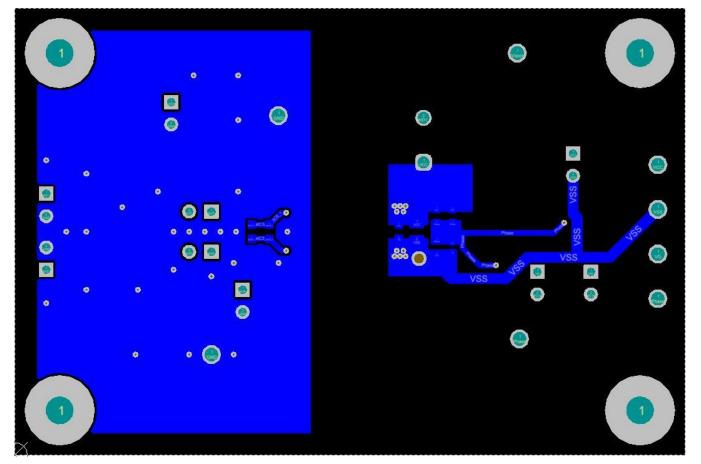
Figure 32. Bottom-Layer Traces and Copper (Flipped)
