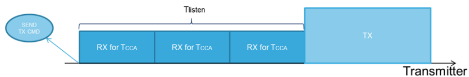
Figure 23. CSMA if channel is free (timeline)
