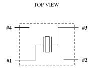
Terminal #2, #4 are connected to the LID (Please connect GND)
