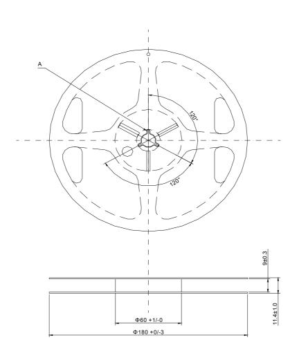
Material:Polystyrene (Conductivity) unit:mm
