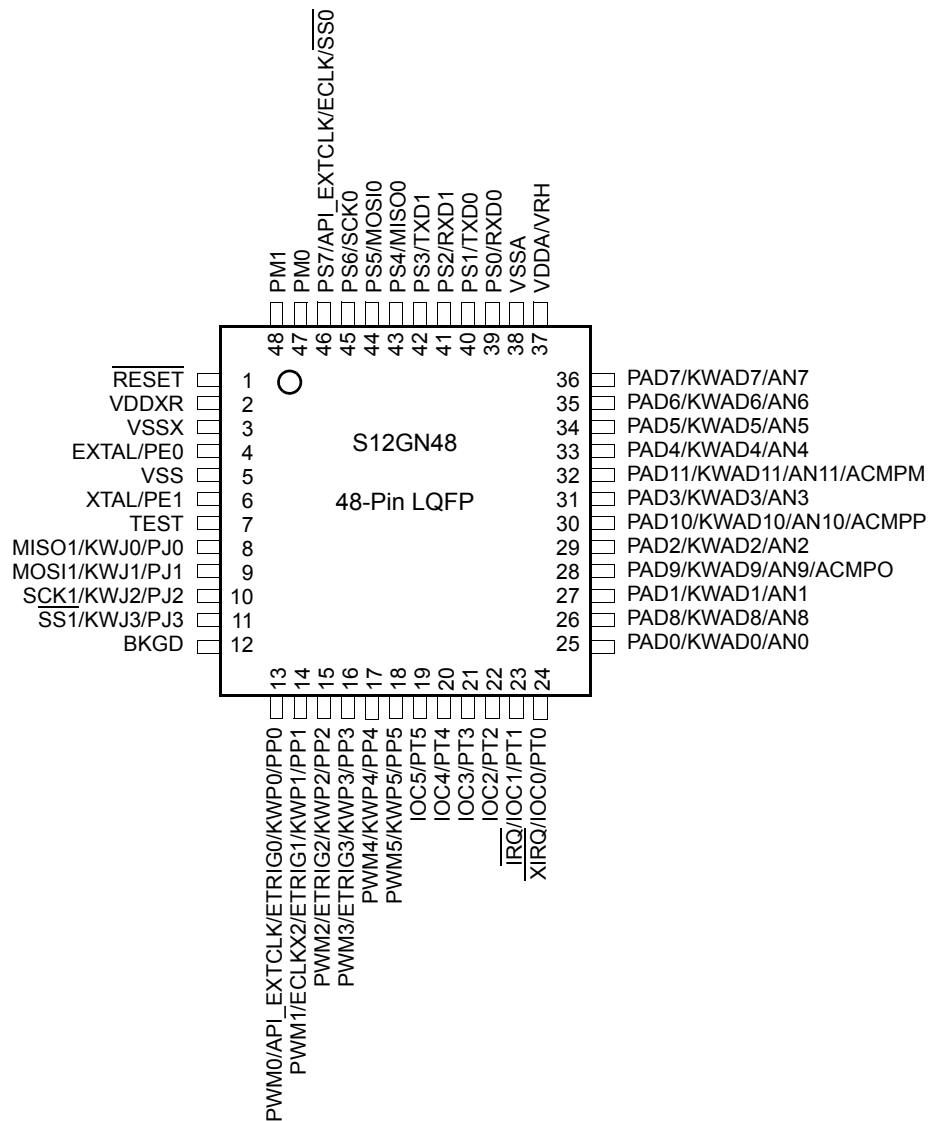
Figure 1-8. 48-Pin LQFP Pinout for S12GN48
