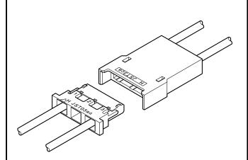
Wire-to-wire version connectors, designed for liquid crystal display back light lamps.
