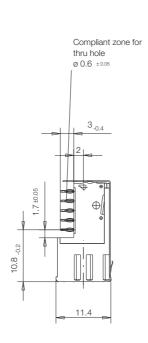
Board hole pattern (Component mounting side)
