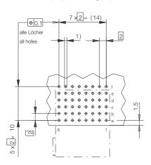
1)  $\emptyset$  0,6±0,05 Diameter of finished plated-through hole  $\emptyset$  0,7±0,02 Diameter of drilled hole
