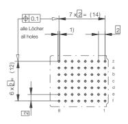
1) ø 0,6±0,05 Diameter of finished plated-through hole ø 0,7  $^{\pm0,02}$  Diameter of drilled hole
