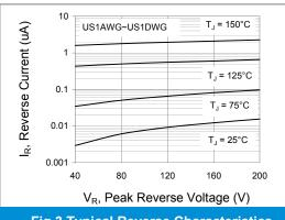
Fig.3 Typical Reverse Characteristics
