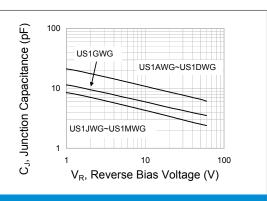
**Fig.2 Typical Junction Capacitance**
