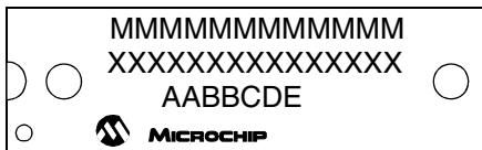
28-Lead PDIP (Skinny DIP)
