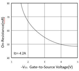
Fig.2 On-Resistance vs. G-S Voltage
