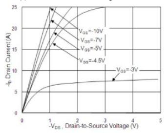
Fig.1 Typical Output Characteristics
