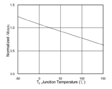
Fig.5 Normalized V GS(th) vs. T J
