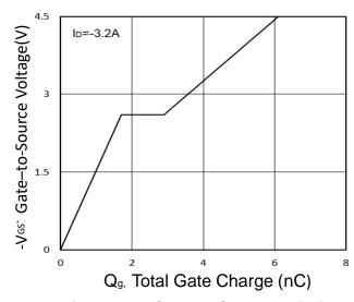
Fig.4 Gate-Charge Characteristics
