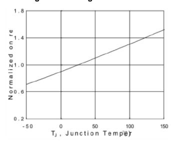
Fig. 6 Normalized R DSON vs. T J
