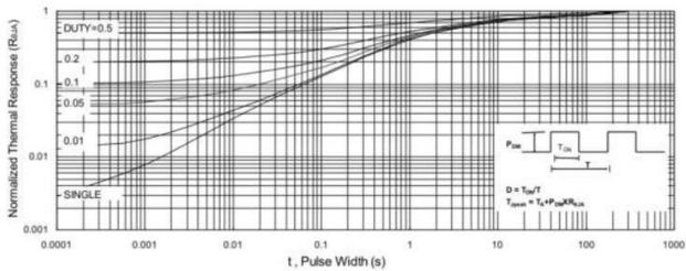
Fig.9 Normalized Maximum Transient Thermal Impedance
