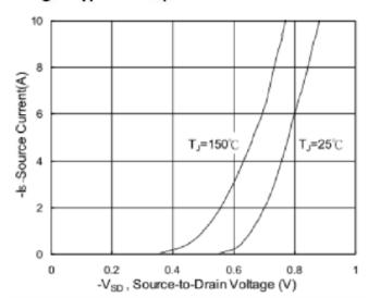
Fig.3 Forward Characteristics of Reverse Diode
