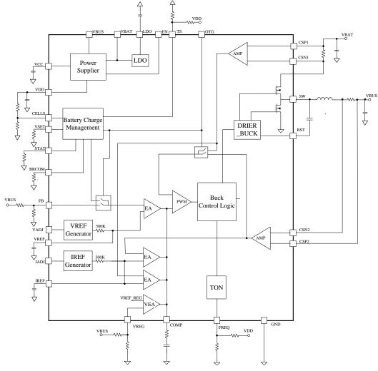
Fig. 22 PL8405 Block Diagram
